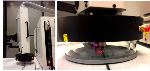
Figure 3. The Temptronic TP4500 with STTS751 temperature sensors under test.
